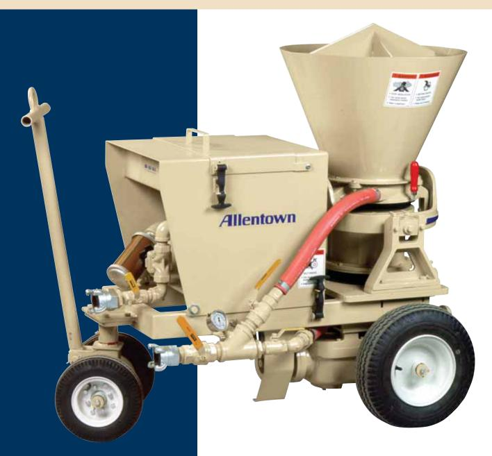
The genuine **Meyco® Piccola** is known around the world. Built by Allentown to the Swiss design, the **Piccola** is a shotcreting machine for processing dry mix using the through-chamber rotor principle. It is versatile, robust, requires little maintenance, and is very easy to operate.
