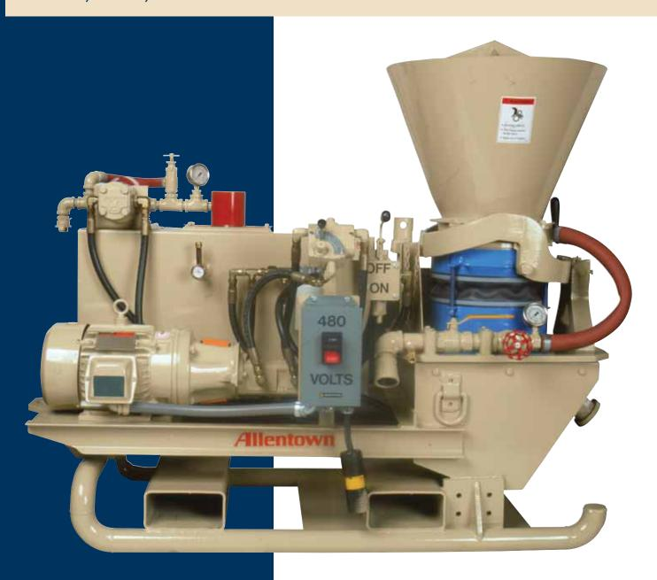
Allentown's **GRH-610 Rotary Gun** is similar to the Meyco Piccola, sharing the same single point clamping system. The use of a compact, efficient, hydrostatic transmission drive gives precise rotor speed with electric, diesel, or gasoline engine power.
